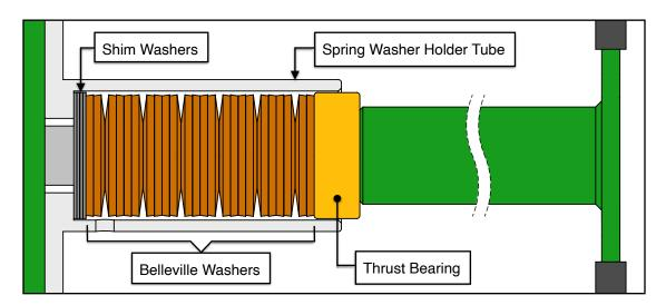
Therefore, "snug" is the first feel of resistance as the loose handle spins in. From this point on every turn made will be compressing the washer stack towards the desired compression total of 5.5-7mm. This will give optimal blade, belt, and bearing life going forward.
